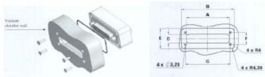
Figure 8 – Dimensions of the hole and mounting description.
